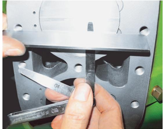
**State of the art reassembly:** Performance must be preserved, here checking the dead volume.
