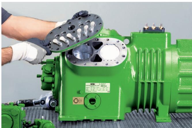
**Professional inspections:** All compressors are completely stripped down. All parts are analysed.
